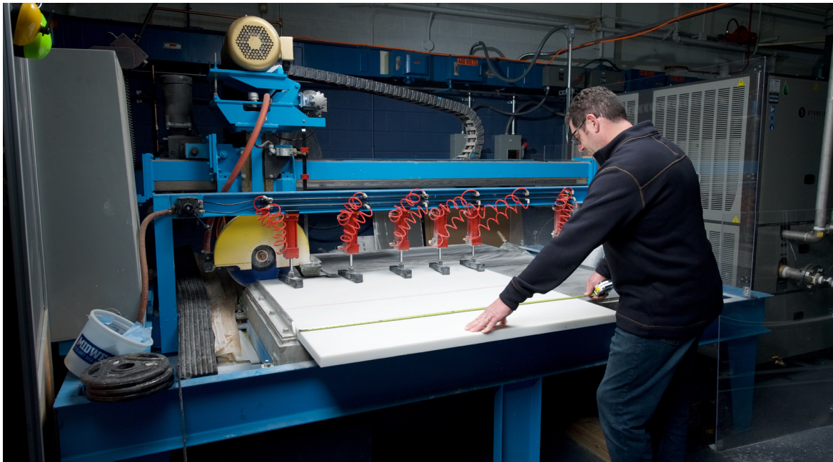
The VAL has a diamond wet saw capable of cutting through silicon ceramic tiles and composite panels
