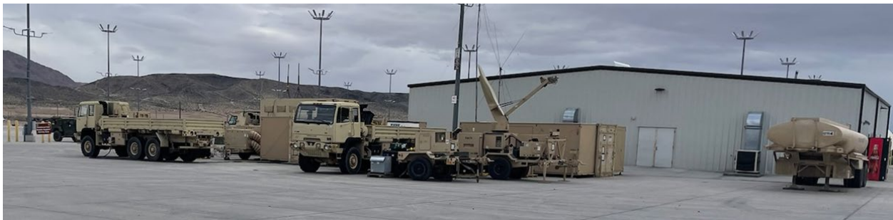
Dual FMTV Vehicle Centric Microgrid supporting three command posts.
